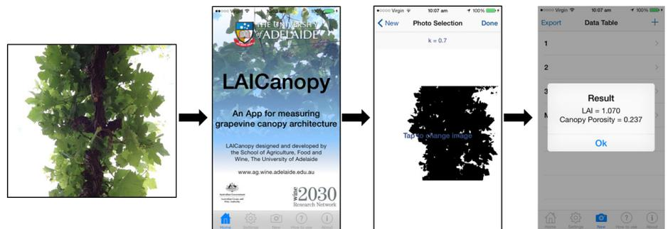
LAICanopy. Upward looking image of a grapevine canopy obtained using an iPad; LAICanopy home page with function tabs; image uploaded to the app and automatically binarised; instant results containing leaf area index (LAI) and canopy porosity.
